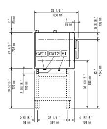
Cold Water inlet 1 (cleaning) CWII Cold Water Inlet 2 (steam CWI2
